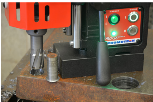
Milling capacity up to 36 mm (1.44") Max depth of cut up to 50 mm (1.97")
